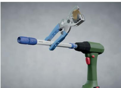
Fig. 19: Calibrating the pipe.
