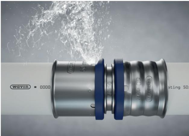
*Fig.14: DEFINED LEAK in the pressure test reveals with leaking water the unpressed fitting.*
